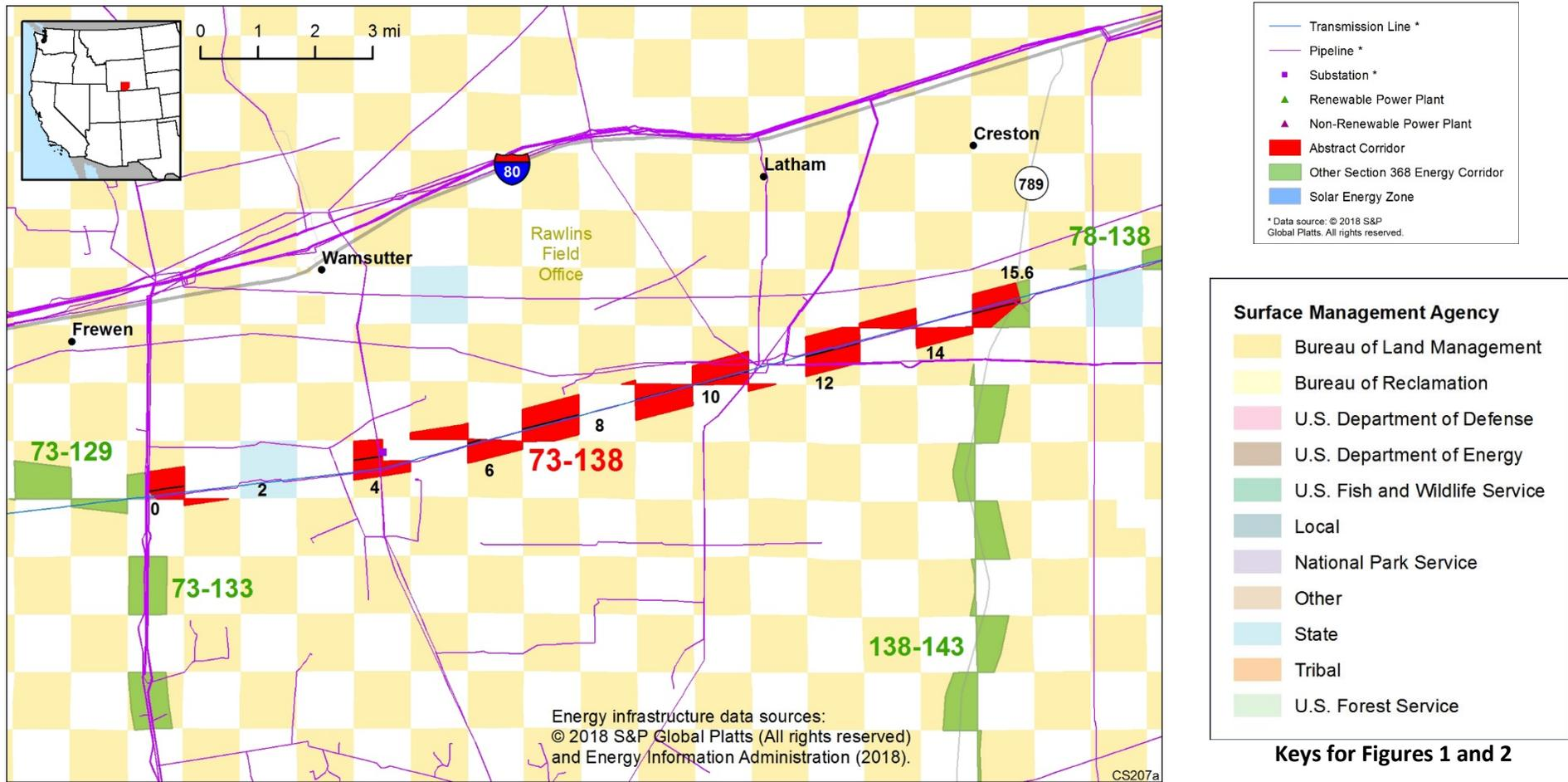
Figure 2. Corridor 73-138 and nearby electric transmission lines and pipelines
