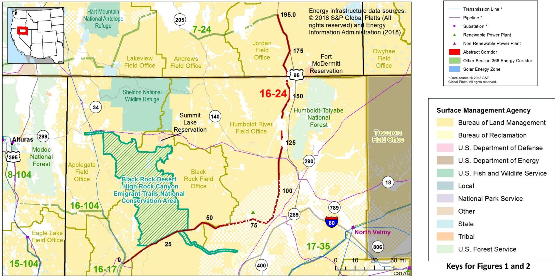
Figure 2. Corridor 16-24 and nearby electric transmission lines and pipelines
