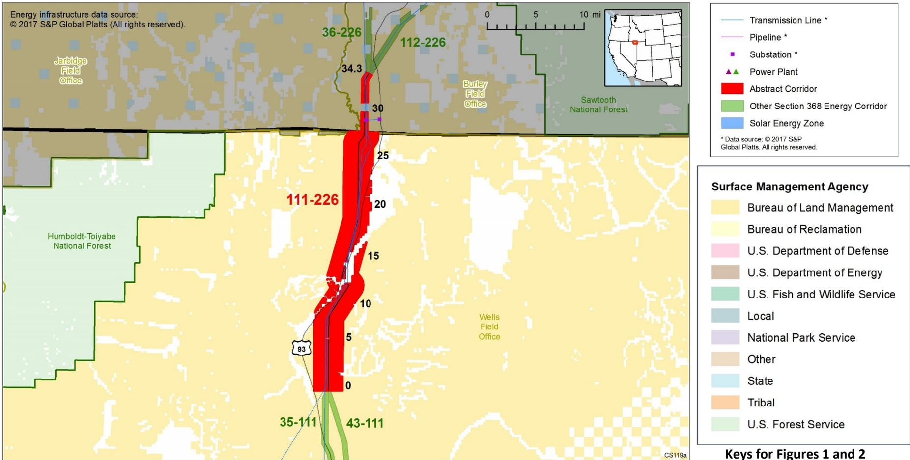
Figure 2. Corridor 111-226 and nearby electric transmission lines and pipelines (grayed out area outside of Region 2 and 3 Review)
